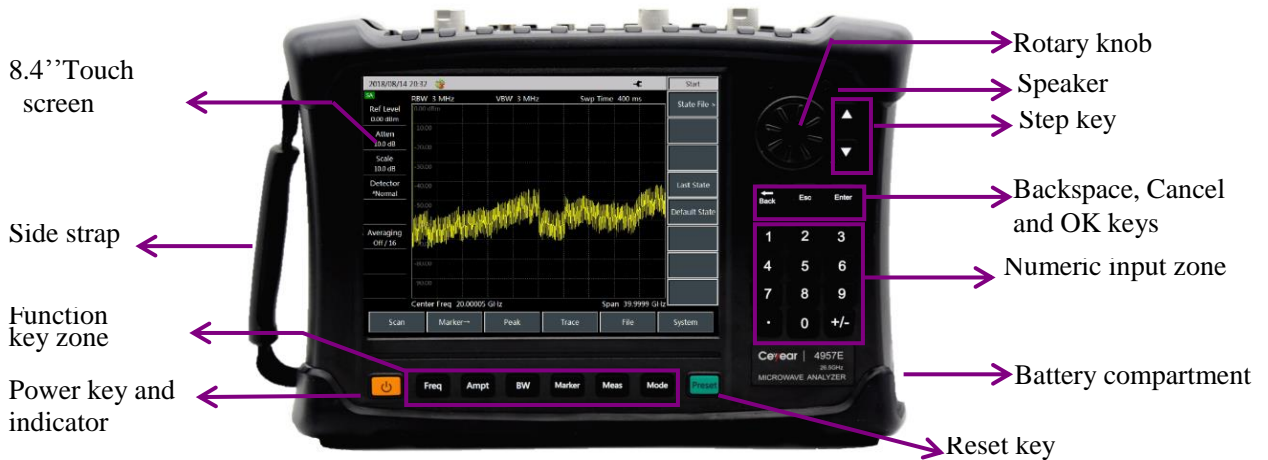
Figure 2.1 Front panel of 4957D/E/F microwave analyzer
