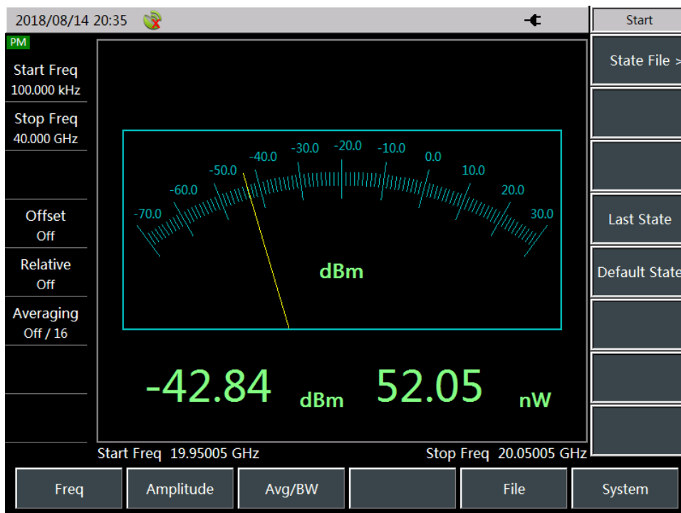
Figure 3.8 Test interface of the PM mode
