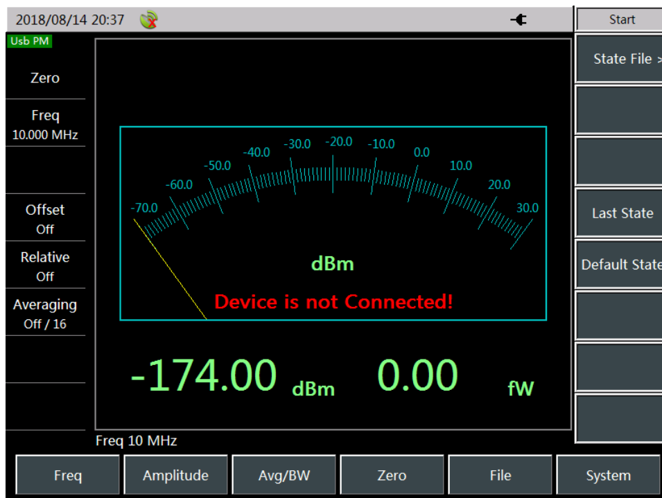
Figure 3.11 Test interface of USB Power Meter mode
